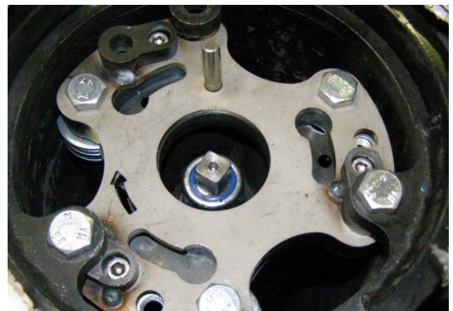
The SP400 'Independence' bollard – picture shows the operating socket on the head of the bollard. This is then covered by a cover.
